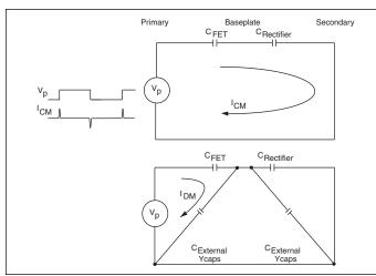
Figure 9-8 — Noise coupling model
